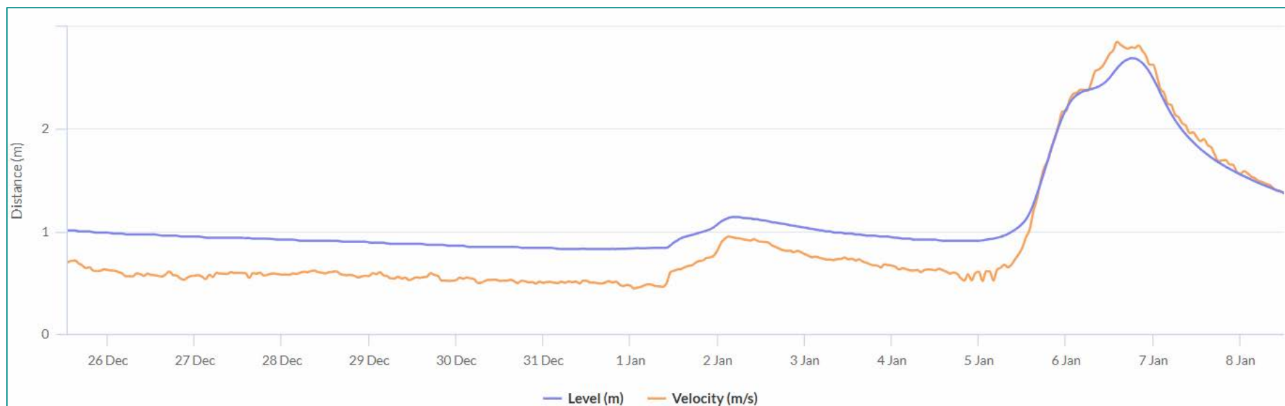
Figure 1: The speed at which Alconbury Brook river height (blue line) responds to rainfall (orange line) 2024/2025 data, taken from recording device in Alconbury Brook
